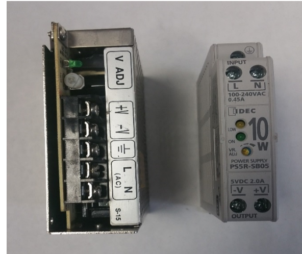
Figure 1 example of 5vdc power supplies
